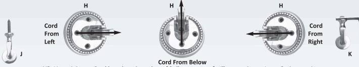
NB Use minimum Cord length and number of Pulleys so as to facilitate optimum Inner Spring tension. Additional Pulleys are available - Please inquire
