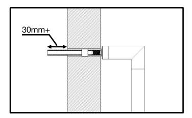
6. If the projection of the bolt from the face of the door is more than 30mm, it may be necessary to shorten the bolts.
