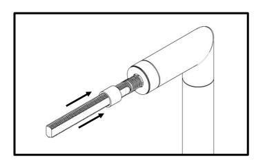
Slide the plastic sleeve (4) over both fixing bolts.
