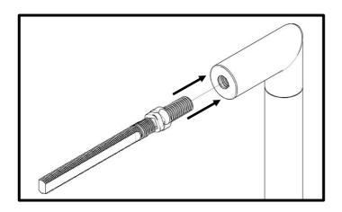
Securely fasten the short screw end of the two fixing bolts (1) onto both ends of the Tubular Handle fixing points.
