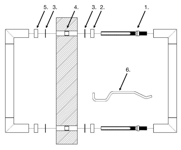
When using this Back to Back Fixing pack you do not require any fixings supplied with the Pull Handle
