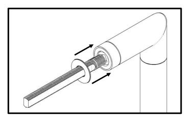
Slide one plastic washer (3) over each of the fixing bolts.
