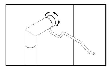
9. Continue to secure the pull handle to the door face by tightening the bush (5) progressively top and bottom until the pull handles are securely fastened to the door.
