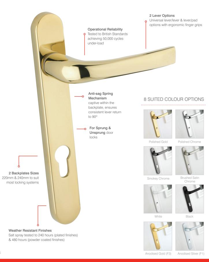
The ProLinea door handle range, designed by Mila's in-house product design team, are suitable for PVCu residential doors. Manufactured from aluminium (painted and anodised finishes) and zinc (plated finishes) the range is available in a choice of eight weather resistant colours.
